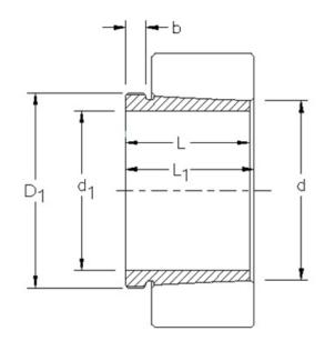
AH3996 Bearing 2D drawings and 3D CAD models
